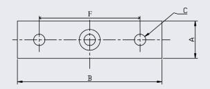
NERO's range of Back Plates are made from 304L stainless steel and come wim a metric tapped boss.
