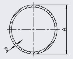
To work out the inside diameter of the pipe
